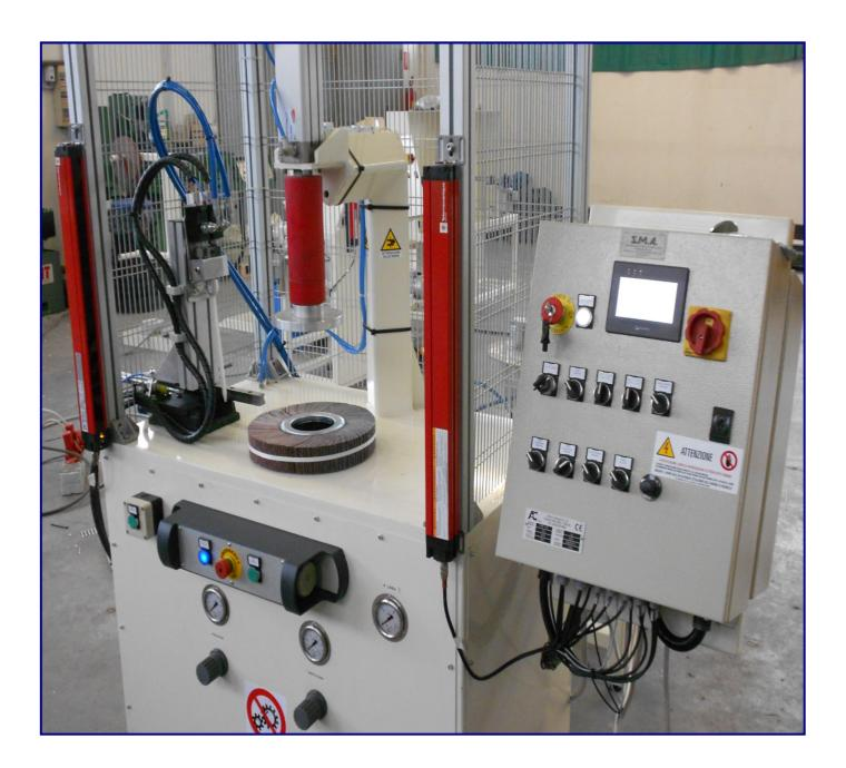
This equipment provides an automatic working process for the pressing of a cloth wheel with flange and the resin coating of its slot. This machine is designed to guarantee a perfect parallelism between the two flanges of the flap wheel and to increase its mechanical resistance due to the gluing of the flanges to the cloth flaps.
